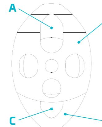
**EN:** (A) Main eyelet, (B) Mobile plate, (C) Symmetric hole, (D) Fixed plate.
